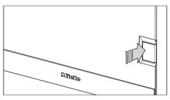
Open the door by pressing on the left hand side of the door release. The door will open slightly.
